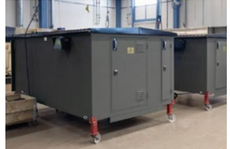
■ Level crossing cabins are prefabricated at Infranord's own workshop. Connecting to the external system is the only thing that remains to be done on delivery.
